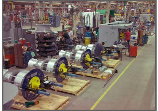
Dynaswirl-LN Burners, Ready for Shipment
